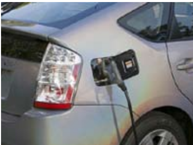
Figure 7. The Toyota Prius is an electric hybrid that provides substantial gains in fuel economy and major reductions in total tailpipe emissions. Reductions in CO 2 emissions will vary depending on the source of the electricity that recharges the secondary battery. It has an energy efficiency of 1.5 passenger-miles per kWh.
