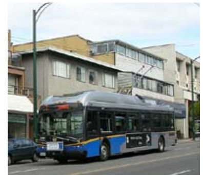
Figure 4. A trolley bus in Vancouver, BC is powered by overhead electrical wires therefore eliminating any tailpipe emissions. The energy efficiency for a trolleybus is approximately 10 passenger-miles per kWh.
