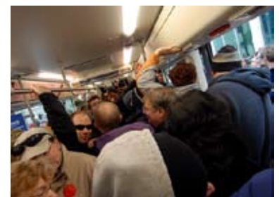
Figure 12. The crush capacity for articulated diesel buses in Vancouver, BC (above) is approximately 100 passengers. Demery & Higgins (2003) found that peak occupancy for buses is less than 3 passengers per meter compared to 4-5 passengers per meter for rail. Below is a picture of a modern streetcar at peak capacity.
